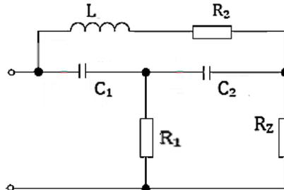
Parametre:  $R_1 = R_2 = 10 \Omega$ ,  $R_z = 10 \text{ k}\Omega$ ,  $L = 10 \text{ mH}$ ,  $C_1 = 10 \mu\text{F}$ ,  $C_2 = 100 \mu\text{F}$ ,  $U_l = 1 \text{ V}$
